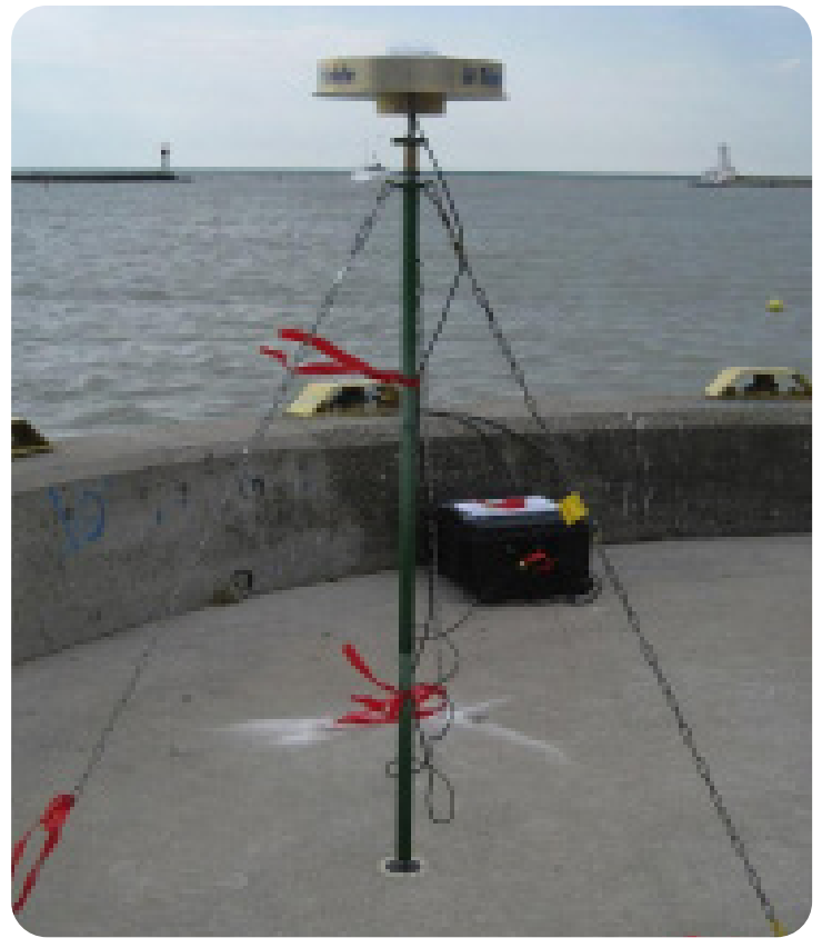
Fig. 3: Typical GNSS set-ups in U.S. and Canada. Image Credit: NRCan.
